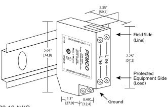
Wire Size Range = 22-12 AWG Terminal Torque Rating = 0.8 Nm (7 in-lb)
